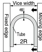
Fix the tube as the left figure shows. Slowly move the moving edge toward the fixed edge. When "a" deforms 25% from the initial value, the measured R is Minimum Installation Radius.
